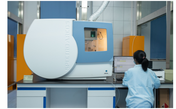
电感耦合等离子体发射光谱仪 Inductively Coupled Plasma Optical Emission Spectrometer
